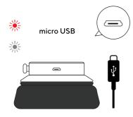
Low battery audible prompts will be announced. Insert micro-USB using a wall charger not computer. Charging LED turns off when fully charged.
