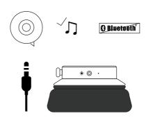
Insert the 3.5mm cable into the port to automatically switch to aux in. HeadSpace does not need to be powered on. If HeadSpace is powered on Bluetooth is disabled to extend battery life.
